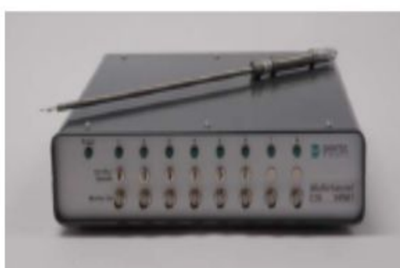
Multichannel CTA with Reference Velocity Transducer
