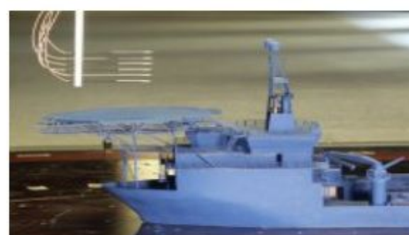
Hot - Wire Probe array measuring on a model of a helicopter landing pad on a ship
