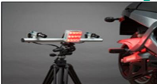
DANTEC Digital Image Correlation System for stress and strain measurement
